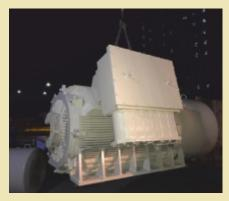
Here's one of the six good-looking 690V large motors that we despatched to a global Heavy Engineering company. The motors range from 250kW to 1000 kW and will be used for their conveyor application at a Coal Terminal in Karnataka.
