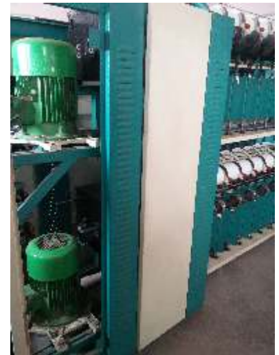
IE4 motors installed and running on TFO textile machines
